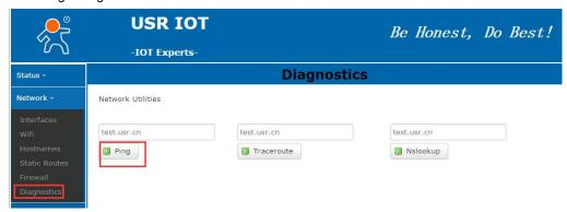
Router's on-line diagnosing function, including Ping tools, route analyzing tools, DNS checking tools.
