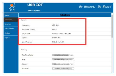
Status page mainly shows device's name information, firmware version, current running state, firewall and routing table display, etc.
