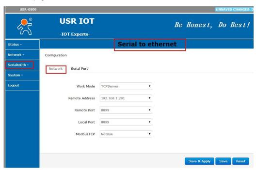
Mainly parameter setting for serial port transforming to network, including working mode, local port, target address, and serial port parameter setting.
