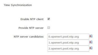
Router can make network timing, default starting NTP Javascript function. There is candidate server address setting.
