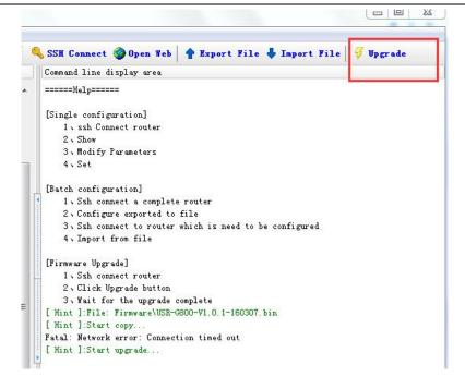
► Export and Import for parameter configuration files. Export and Import configuration files are under "Root Directory/etc/config"
