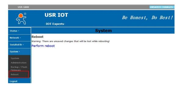
Click the button to restart the router. Restarting time is same as router's power on starting time, completely and successfully start after about 30-40 seconds.
